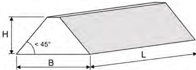
Abb. 40: Grundform eines Sandsackdamms (BABS)
