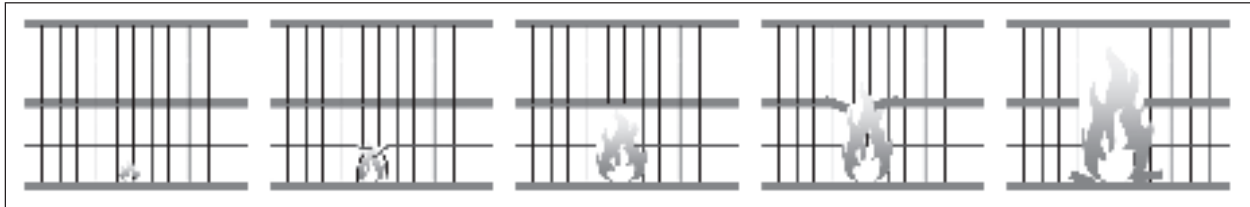
Fig. 9: How a fire could develop and cause massive internal collapse at the National Library of Scotland. After a short time, the flames may spread over four floors, penetrating one solid floor and two intermediate floors.
